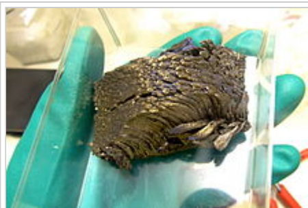
About 300 g of dendritic sublimated 99.998% pure europium handled in a glove box
