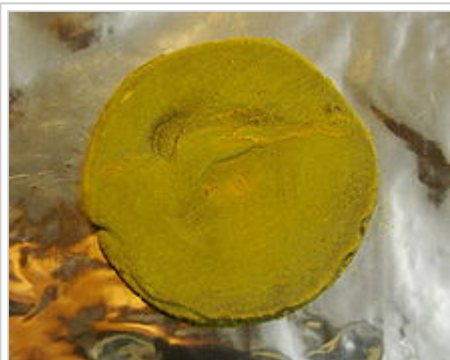
Oxidized europium, coated with yellow europium(II) carbonate
